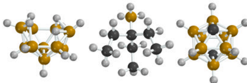
Figure 12 The dependence of the sulfuraceous character on molecular vibrations and atomic partial charges, as predicted by a vibrational theory. Decaborane (left) smells sulfuraceous, and its terminal B-H bonds have a stretch frequency \sim 2500 wavenumbers. In triethylamine-borane (middle), the B-H stretch is shifted to 2300 wavenumbers and the sulfuraceous smell is no longer present. In p-carborane (right) the near-neutral partial charges make the SH bond odorless.
